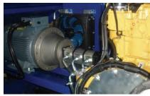
Dual Power -Provides two running options; Diesel / hyd. or Electric/ hyd.
