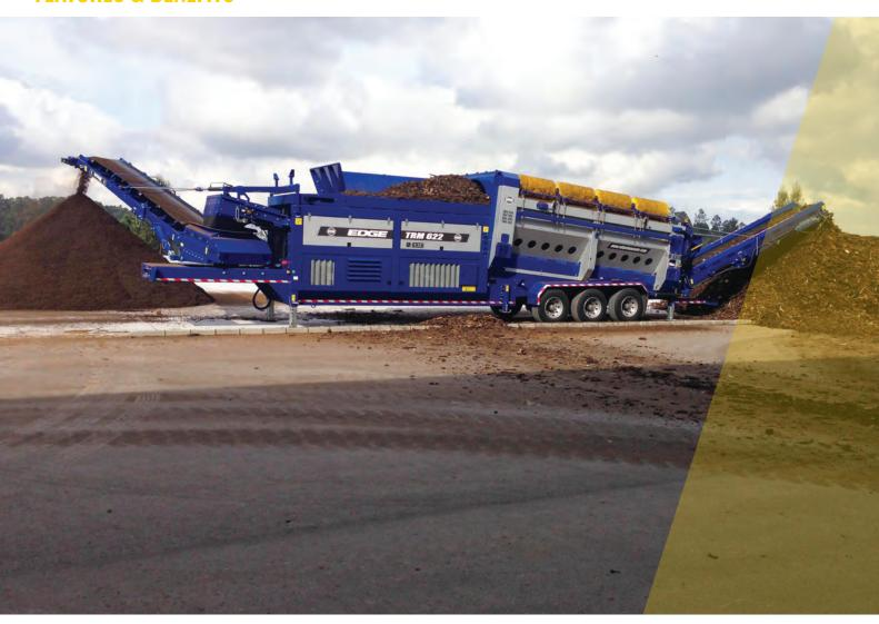
The EDGE TR622 Trommel Series combines high production rates with ease of use in a robust, portable and versatile screening plant that is ideal for applications such as top soil, recycling, composting and is proven in construction and demolition waste.
