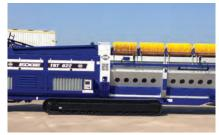
Tracked Mounted - Fully tracked for on-site manoeuvrability
